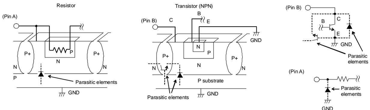
Fig.29 Example of a Simple Monolithic IC Architecture
