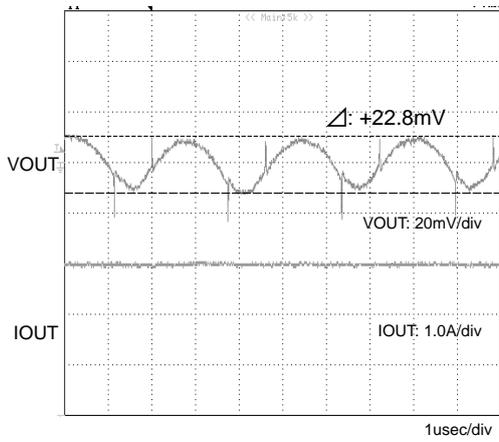
Fig.16 Output Ripple Voltage
