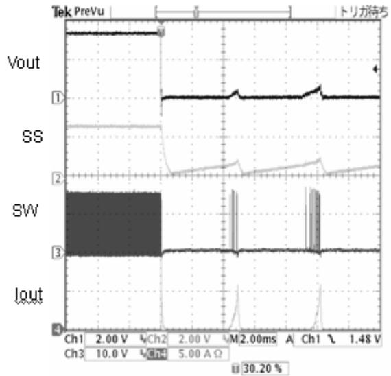
Fig.11 OverCurrent Protection
