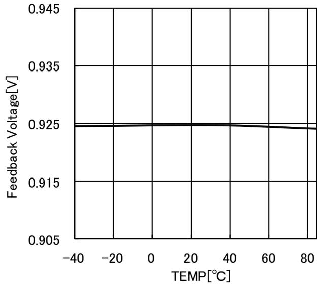
Fig.7 Feedback voltage
