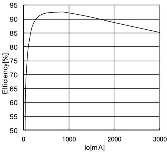
Fig.10 STEP Down Efficiency
