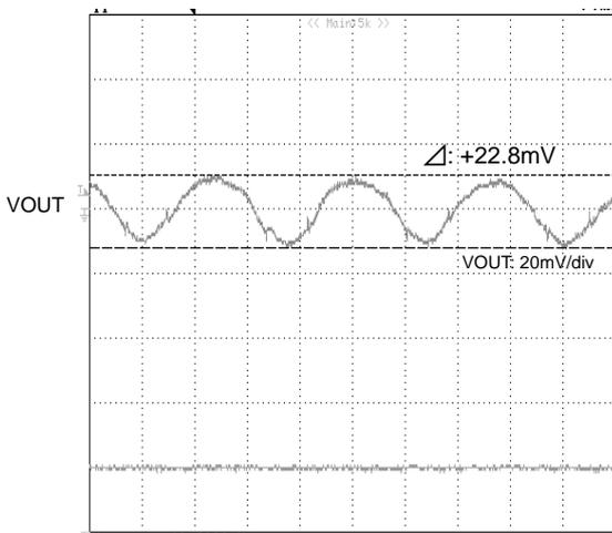
Fig.14 Output Ripple Voltage
