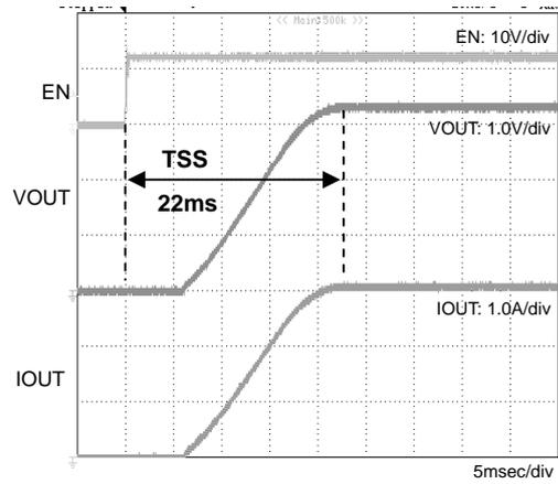
Fig.17 Start Up waveform
