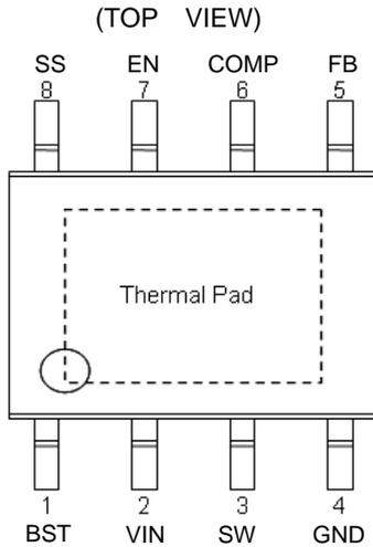
Fig.2 Pin Configuration
