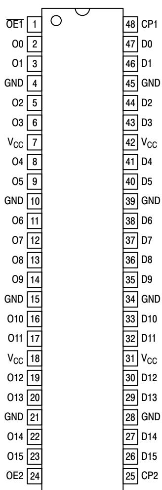
**Figure 1. Pinout: 48-Lead
