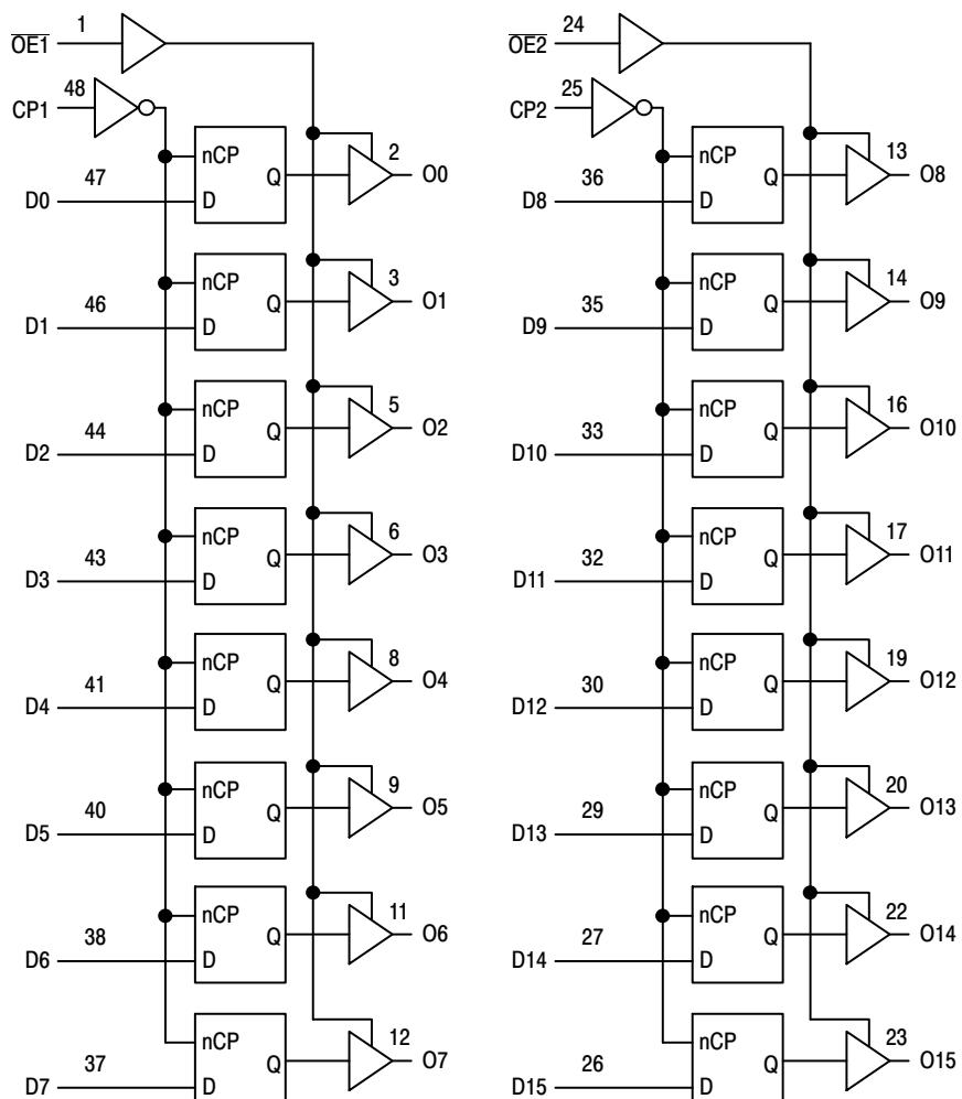
**Figure 2. Logic Diagram**
