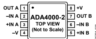
Figure 4. 8-Lead MSOP (RM-8)
