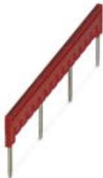
Plug-in bridge, non-adjacent, Pitch: 8.2 mm, Number of positions: 16, Pin assignment: 1, 6, 11, 16, Color: red
