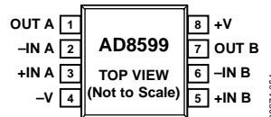
Figure 3. AD8599 8-Lead SOIC (R-8)
