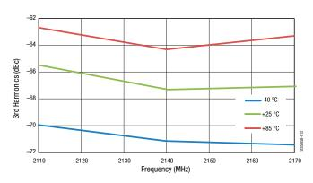
Figure 12. 3rd Harmonic @ +28 dBm vs Frequency Across Temperature
