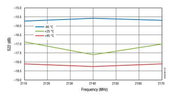
Figure 18. Output Return Loss vs Frequency Across Temperature (Small Signal, PiN = -30 dBm)
