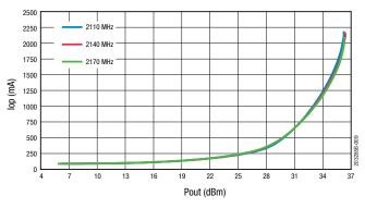
Figure 9. IOP vs Pout Across Frequency
