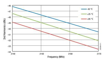
Figure 11. 2nd Harmonic @ +28 dBm vs Frequency Across Temperature
