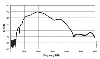
Figure 13. Gain vs Frequency (Small Signal, Pin = -30 dBm)
