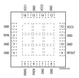
Figure 2. SKY66294-11 Pinout (Top View)
