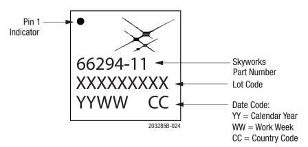
Figure 24. Typical Part Marking for the SKY66294-11
