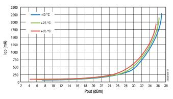
Figure 10. lop vs Pout Across Temperature
