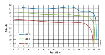
Figure 7. Gain vs Pout Across Frequency
