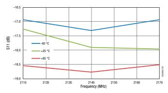
Figure 16. Input Return Loss vs Frequency Across Temperature (Small Signal, PIN = -30 dBm)
