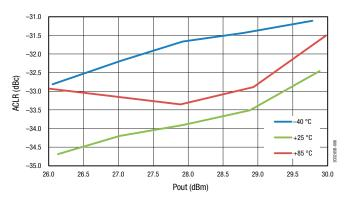
Figure 5. ACLR vs Pout Across Frequency (20 MHz LTE, 8.5 dB PAR Signal)
