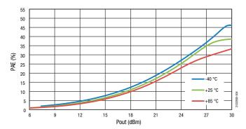
**Figure 3. PAE vs Pout Across Frequency**
