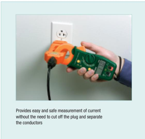
Provides easy and safe measurement of current without the need to cut off the plug and separate the conductors
