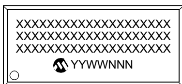
28-Lead SOIC (7.50 mm)
