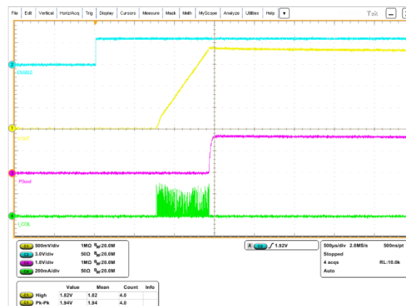
Figure 16. Start-up, V_{IN}=3.6\text{ V} , V_{OUT}=1.8\text{ V} , no load
