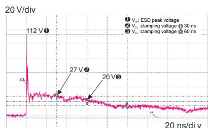
**Figure 8.** ESD response to IEC 61000-4-2 (-8 kV contact discharge)
