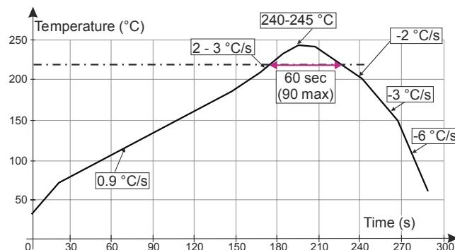
Note: Minimize air convection currents in the reflow oven to avoid component movement.
