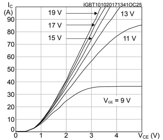
**Figure 5. IGBT transfer characteristics**
