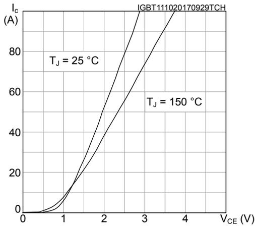
**Figure 4. IGBT output characteristics**
