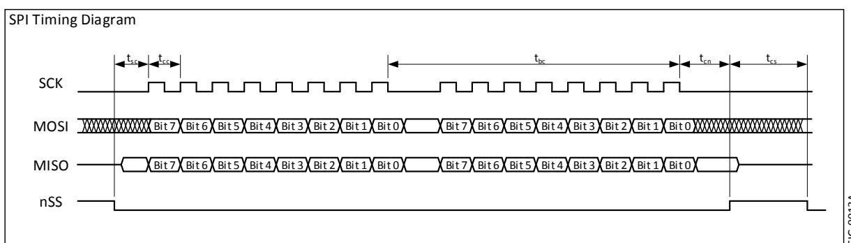
The data communications has been reduced to a simple 16 bit transfer model for reading the pressure output. Each communication cycle consists of master sending the Mode and Rate data to be placed into the sensor Mode Register and Rate Registers respectively. Simultaneously, the sensor sends the pressure data for the master to receive. Refer to the figure below for the data communication model of the SP Series sensor.
