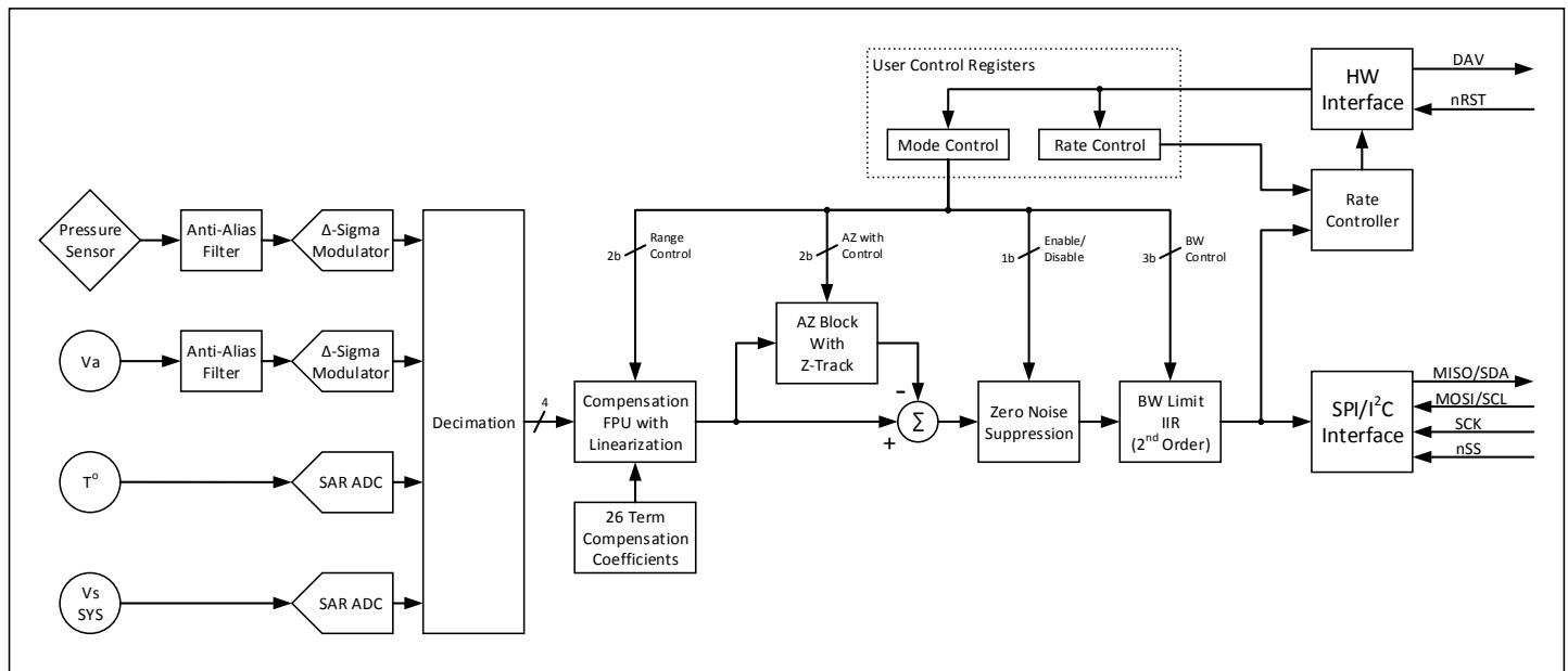
There are also two user controlled registers that tune the sensor to the specific user requirements. The first register is the Mode Control register that determines the output pressure range, the corner frequency of the bandwidth limiting filter, enables or disables the noise suppression filter and controls the Auto-Zero block with Z-Track™.
