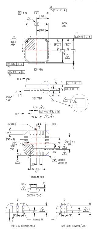
L28.6x6 28 LEAD QUAD FLAT NO-LEAD PLASTIC PACKAGE (COMPLIANT TO JEDEC MO-220VJJC ISSUE C)
