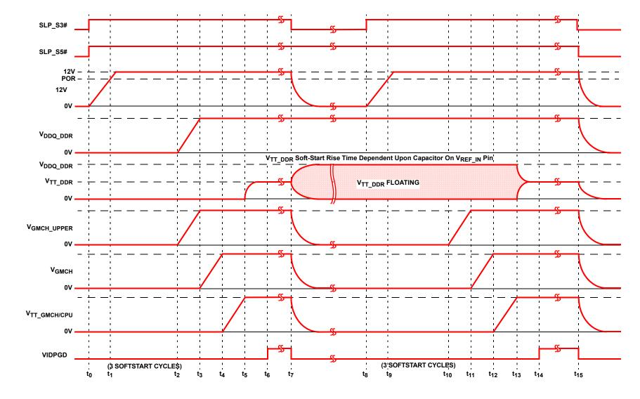
FIGURE 1. ISL6537 TIMING DIAGRAM
