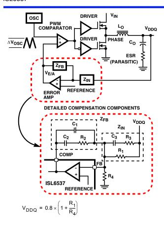
FIGURE 3. VOLTAGE-MODE BUCK CONVERTER
