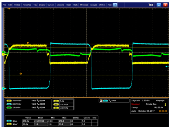
Figure 75 Effect of different values of R_{G,on} on CFD7 switching behavior at I_{out} = 10 \text{ A} . V_{ds} (blue); V_{gs} (yellow); primary current (green).
