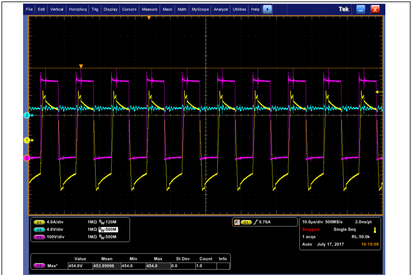
Figure 68 Start-up under short-circuit conditions. Primary current (yellow), V_{DS} of low-side MOSFET (purple) and output voltage of converter (blue).
