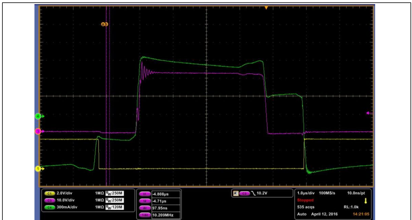
Figure 39 Synchronous MOSFET gate pulse (yellow), V_{DS} (purple) and primary current of the transformer (green)
