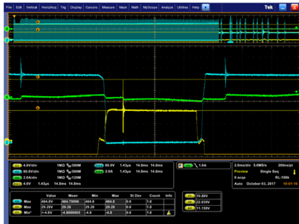
Figure 74 Effect of different values of R_{G,on} on CFD7 switching behavior during start-up at no load. V_{ds} (blue); V_{gs} (yellow); primary current (green).
