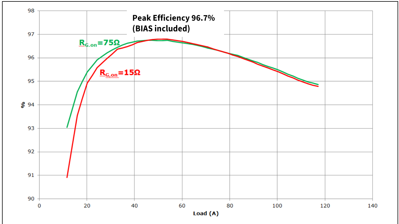
Figure 76 Effect of different values of R_{G,on} on IPP60R170CFD7 efficiency plot in 1400 W demo board
