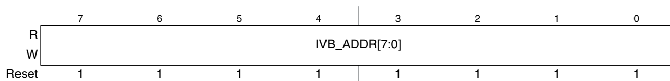
Figure 6-2. Interrupt Vector Base Register (IVBR)
