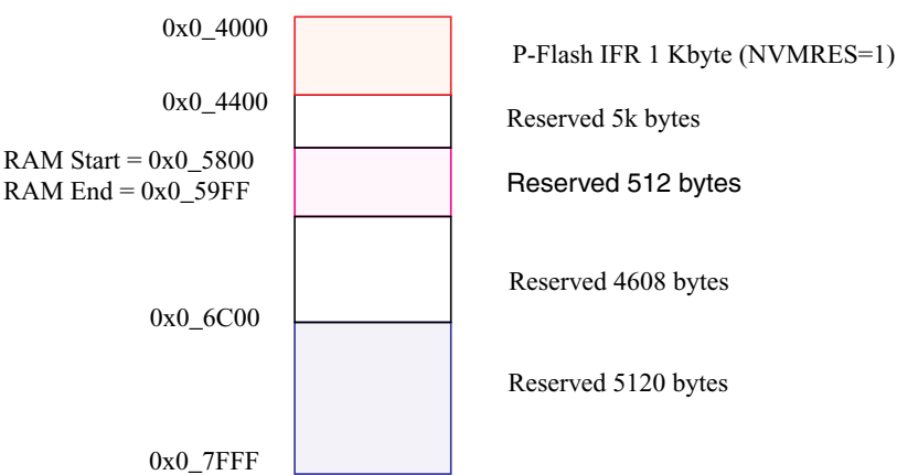
Figure 24-3. Memory Controller Resource Memory Map (NVMRES=1)
