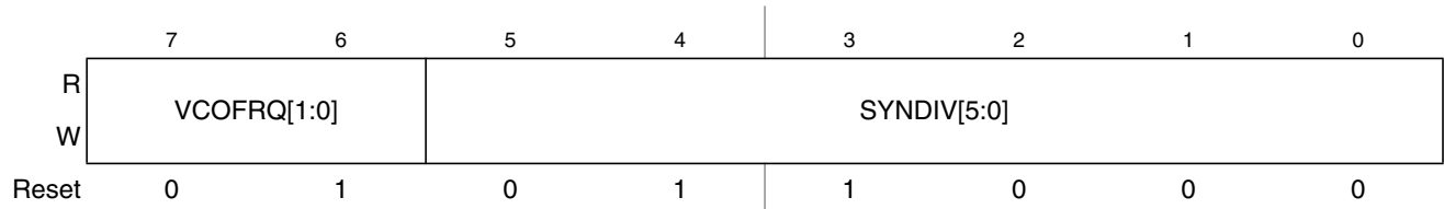
Figure 10-4. S12CPMU Synthesizer Register (CPMUSYNR)
