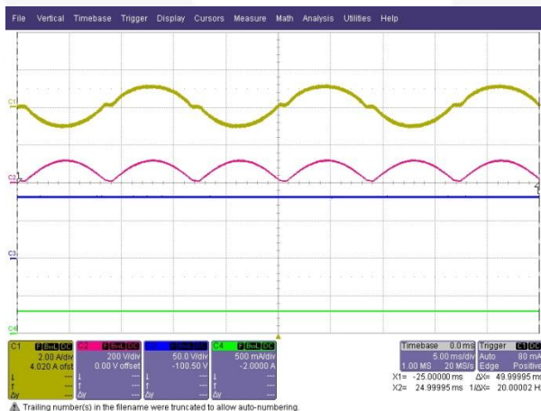
Figure 39. V IN = 85 V AC / 60 Hz, 50% Dim
