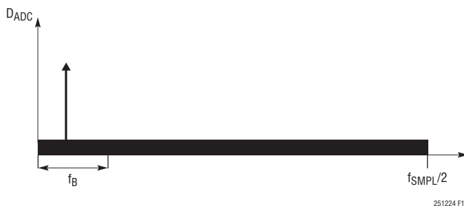
Figure 15. Frequency Spectrum of SAR ADC Core Output
