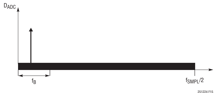
Figure 15. Frequency Spectrum of SAR ADC Core Output
