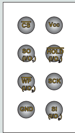
Figure 1-3. 8-ball WLCSP (Bottom View)
