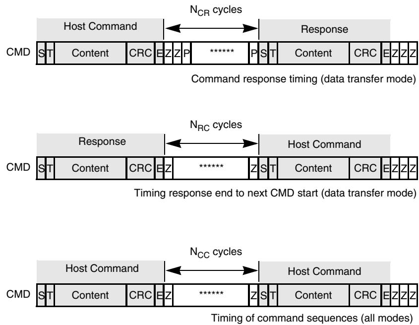
**Figure 49. Timing Diagrams at Data Transfer Mode**
