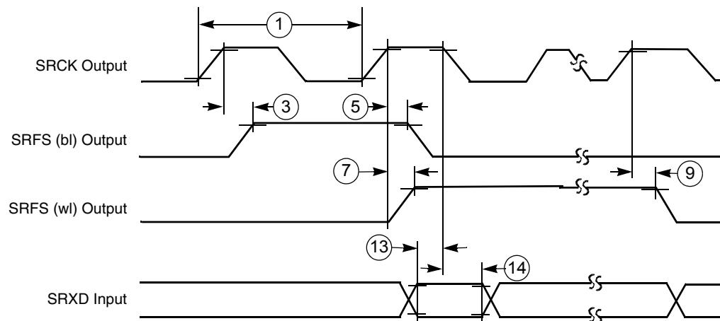
**Figure 65. SSI Receiver Internal Clock Timing Diagram**
