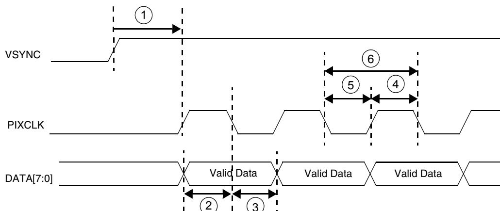
**Figure 71. Sensor Output Data on Pixel Clock Rising Edge
