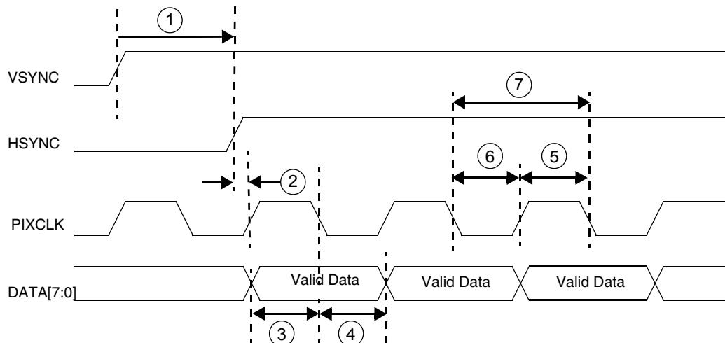
**Figure 69. Sensor Output Data on Pixel Clock Rising Edge
