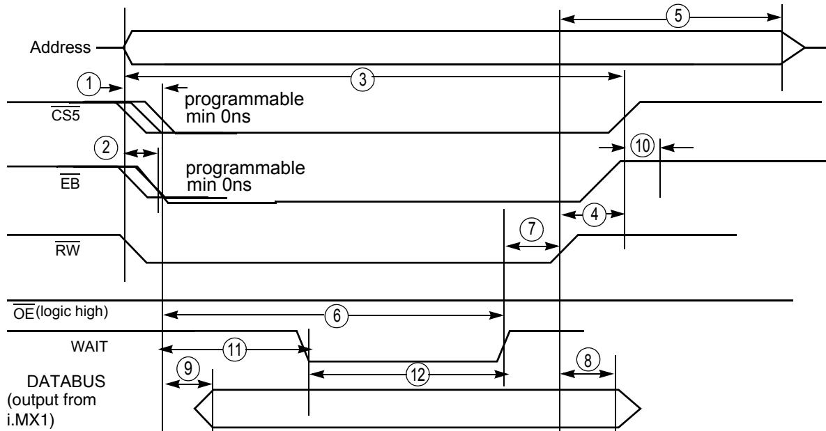
**Figure 8. WAIT Write Cycle without DMA****Table 15. WAIT Write Cycle without DMA: WSC = 111111, DTACK\_SEL=1, HCLK=96MHz**
