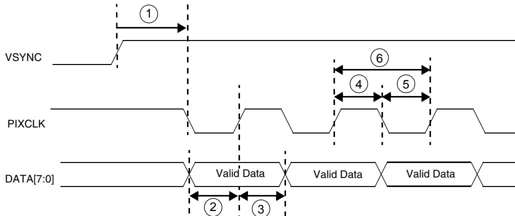
**Figure 70. Sensor Output Data on Pixel Clock Falling Edge
