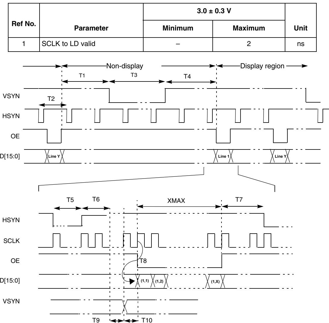
**Figure 46. 4/8/16 Bit/Pixel TFT Color Mode Panel Timing****Table 27. 4/8/16 Bit/Pixel TFT Color Mode Panel Timing**
