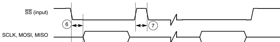
**Figure 43. Slave SPI Timing Diagram FIFO Advanced by SS Rising Edge**
