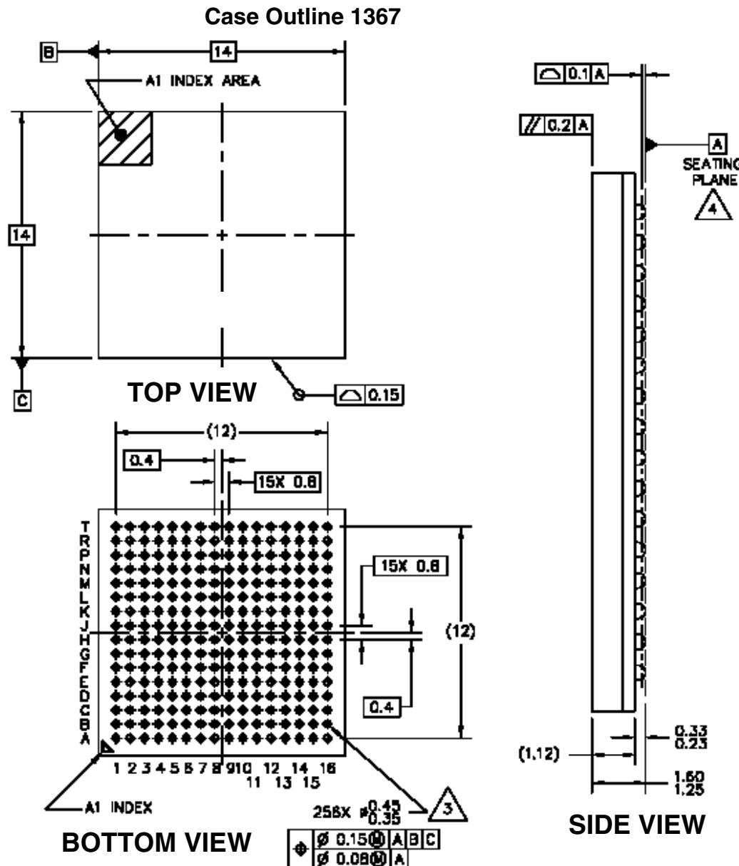
Figure 72. i.MXL 256 MAPBGA Mechanical Drawing
