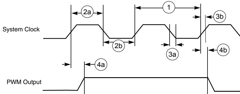
**Figure 56. PWM Output Timing Diagram****Table 32. PWM Output Timing Parameter Table**
