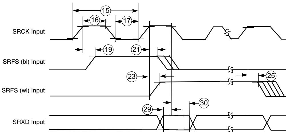
Figure 67. SSI Receiver External Clock Timing Diagram
