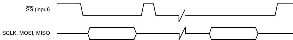
**Figure 42. Slave SPI Timing Diagram FIFO Advanced by BIT COUNT**
