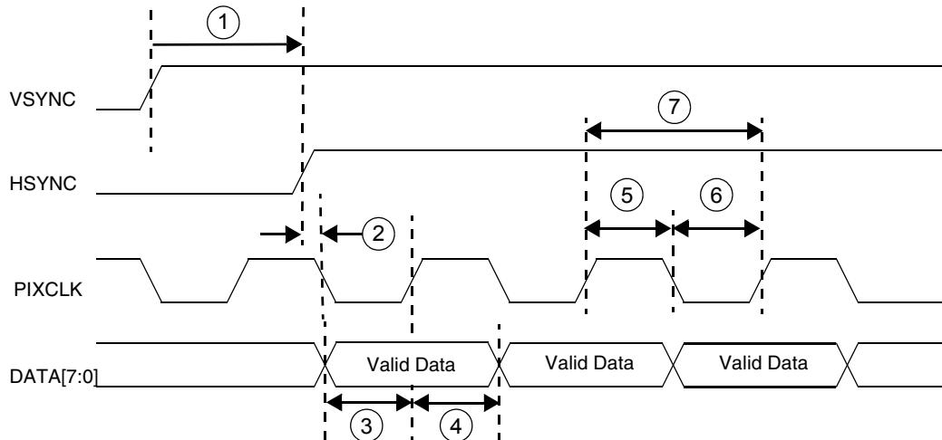
Figure 68. Sensor Output Data on Pixel Clock Falling Edge
