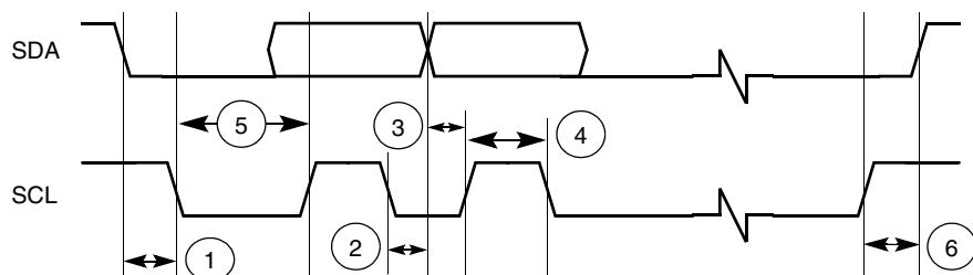
Figure 63. Definition of Bus Timing for I<sup>2</sup>C
