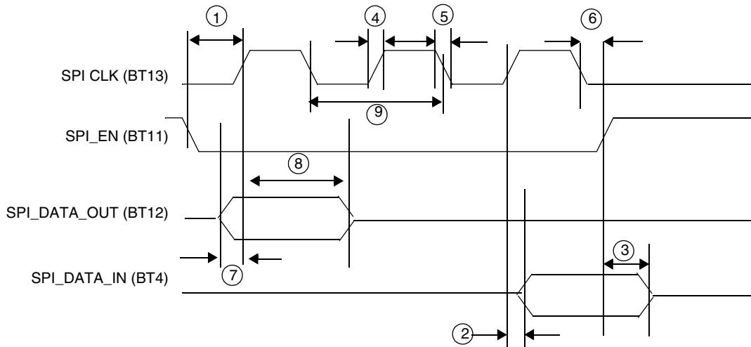
Figure 38. SPI Interface Timing Diagram Using MC13180
