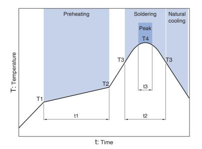
Preheating Soldering Peak Temp. Time Temp. Time Temp. Time **T1** T2 t1 тз t2 Т4 t3 150°C 180°C 60 to 120s 230°C 30s 260°C 10s
