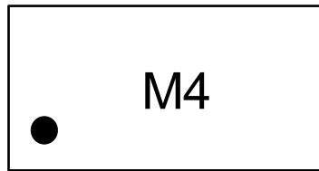
Note: The marking codes can be rotated by 90 ° or 180 ° to differentiate assembly location. In no case should this product marking be used to orient the component for its placement on a PCB. Only pin 1 mark is to be used for this purpose
