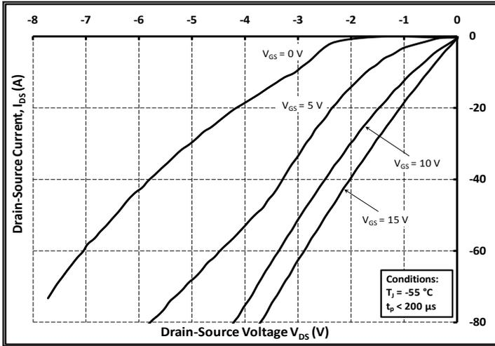
Figure 13. 3rd Quadrant Characteristic at -55 °C
