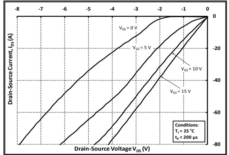
Figure 14. 3rd Quadrant Characteristic at 25 °C
