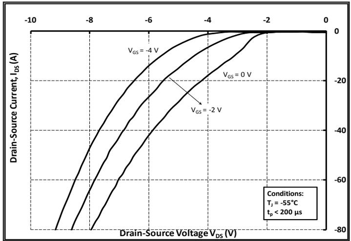
Figure 8. Body Diode Characteristic at  $-55\text{ }^\circ\text{C}$
