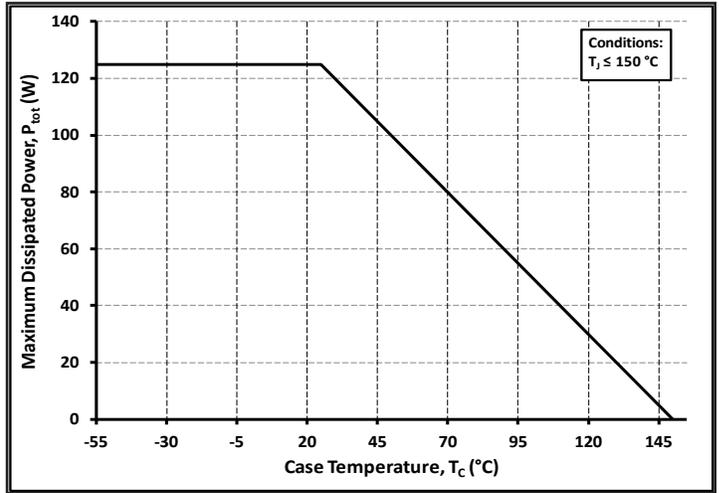
Figure 20. Maximum Power Dissipation Derating vs. Case Temperature
