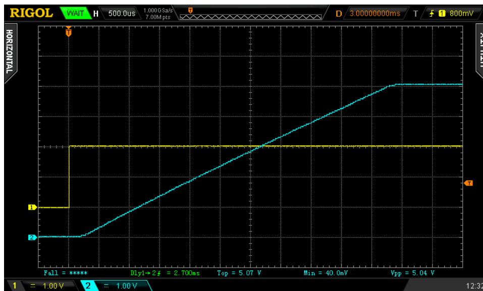
Figure 3. A SLG59M1717V with C_{SLEW} set to 15nF and 470 \mu F retained for C_{LOAD} . C_{LOAD} -to- C_{SLEW} ratio is smaller than 33,600. Note smooth V_{OUT} transition.
