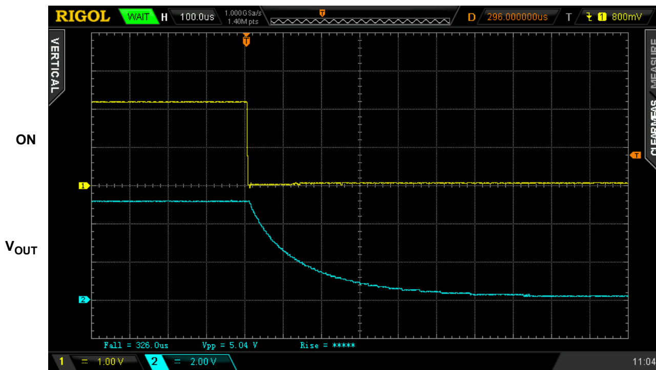
Figure 4. Typical Turn OFF operation waveform for V_{DD} = V_{IN} = 5\text{ V} , C_{SLEW} = 12\text{ nF} , C_{LOAD} = 10\text{ }\mu\text{F} , R_{LOAD} = 20\text{ }\Omega
