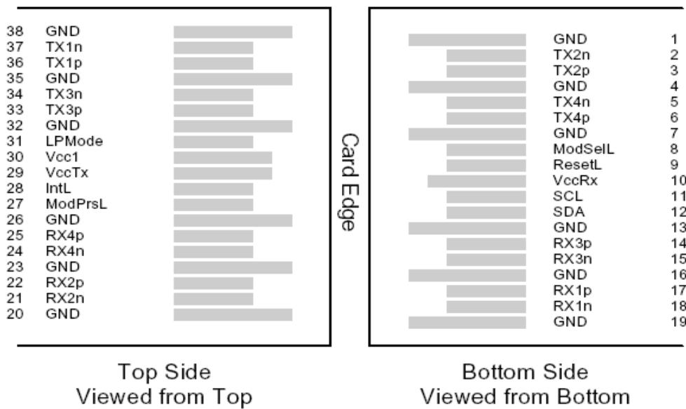
Figure 1 – QSFP28-compliant 38-pin connector (per SFF-8679)
