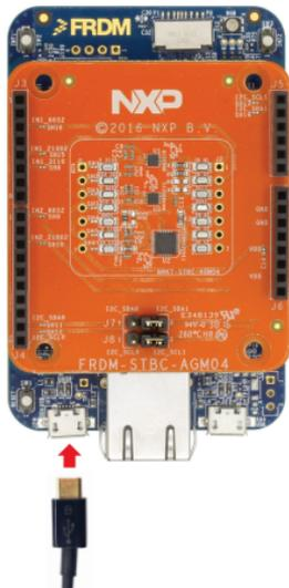
Figure 2: Connect board to computer
