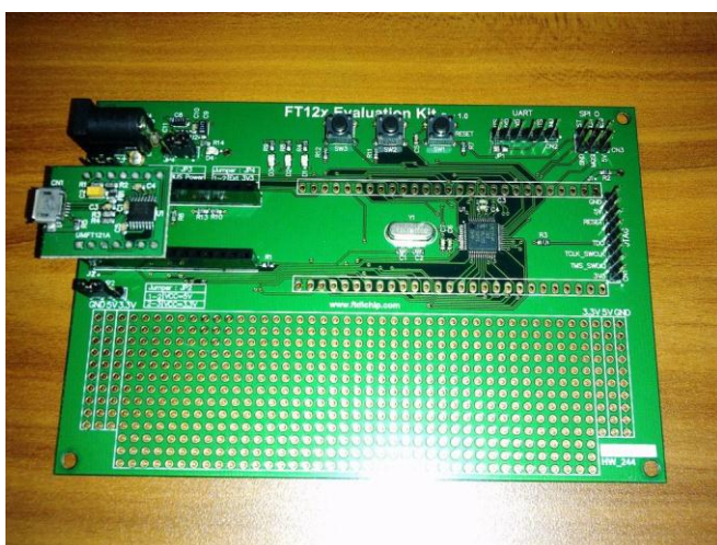
Figure 4-1 Plug the daughter board module to the main board
