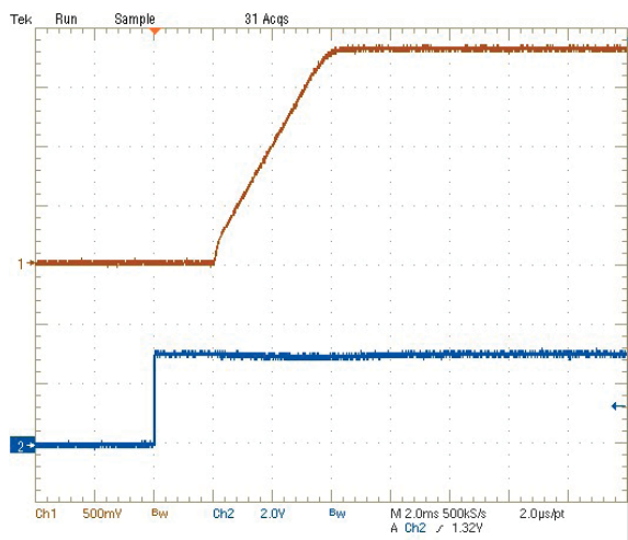
Step Load Transient Response (Vin=5.0V, Vout=1.2V, Cload=94µF, Iout=6A to 12A) Trace 1=Vout, 200 mV/div, Trace 4=Iout, 10A/div.
