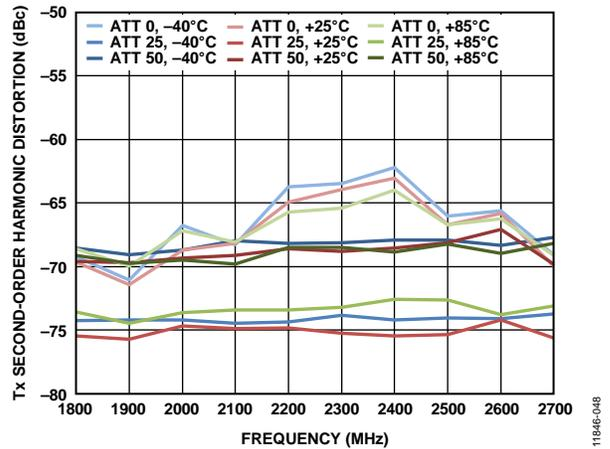
Figure 48. Tx Second-Order Harmonic Distortion (HD2) vs. Frequency
