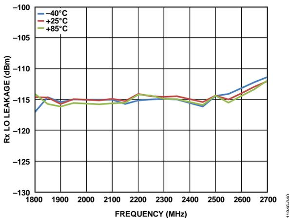
Figure 40. Rx Local Oscillator (LO) Leakage vs. Frequency
