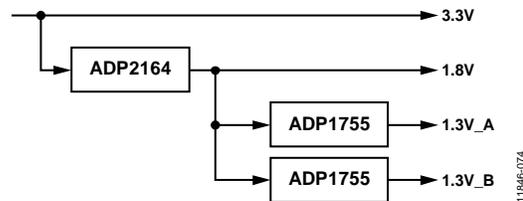
Figure 74. Low Noise Power Solution for the AD9364
