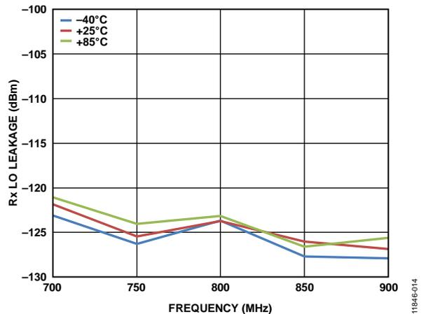
Figure 14. Rx Local Oscillator (LO) Leakage vs. Frequency
