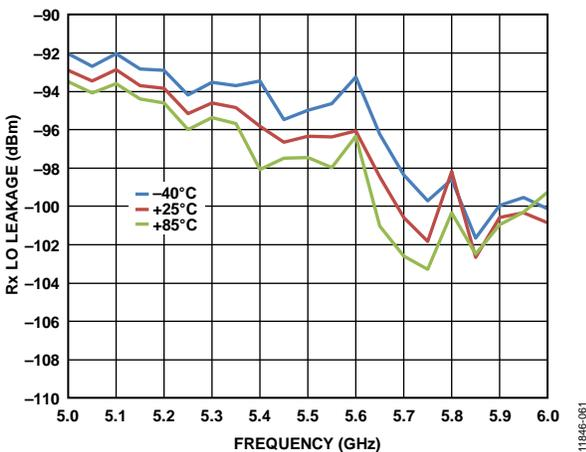
Figure 61. Rx Local Oscillator (LO) Leakage vs. Frequency
