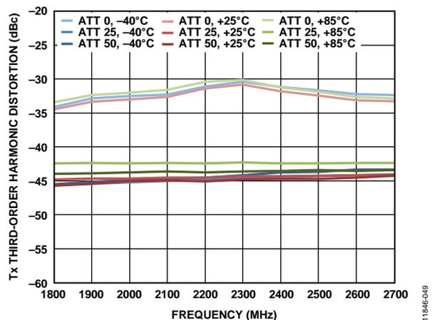
Figure 49. Tx Third-Order Harmonic Distortion (HD3) vs. Frequency
