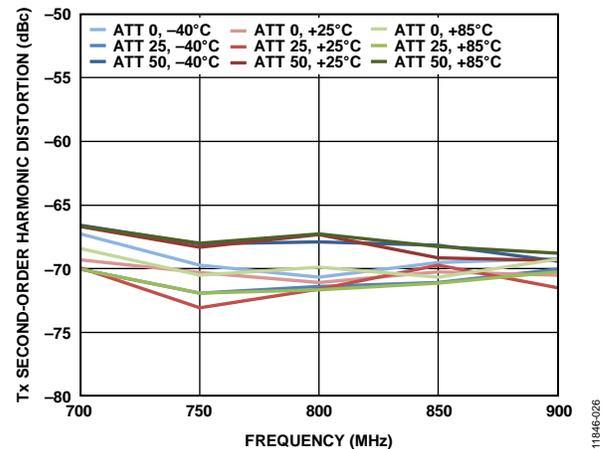
Figure 26. Tx Second-Order Harmonic Distortion (HD2) vs. Frequency
