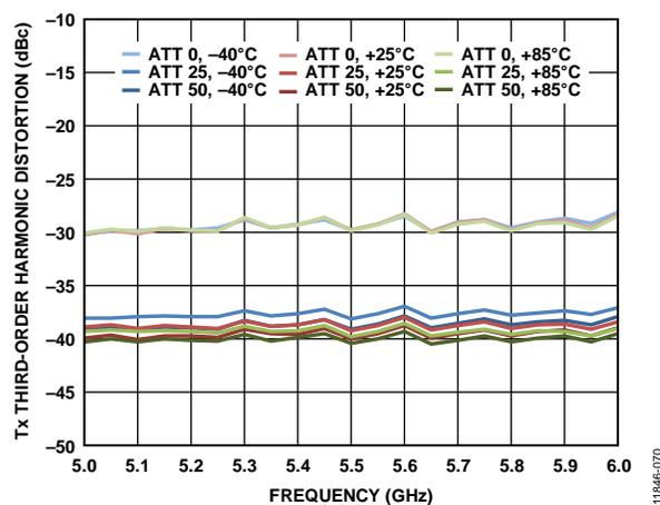
Figure 70. Tx Third-Order Harmonic Distortion (HD3) vs. Frequency
