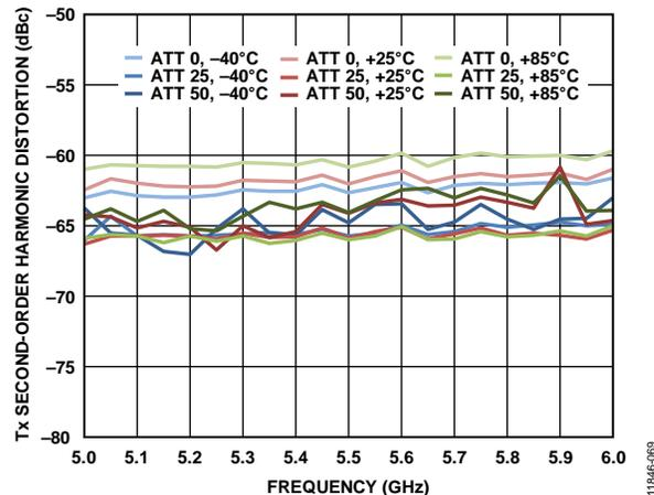
Figure 69. Tx Second-Order Harmonic Distortion (HD2) vs. Frequency
