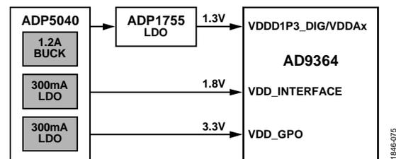
Figure 75. Space-Optimized Power Solution for the AD9364
