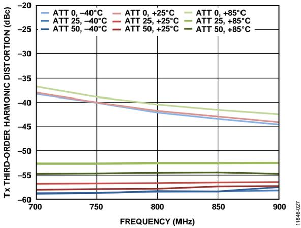
Figure 27. Tx Third-Order Harmonic Distortion (HD3) vs. Frequency
