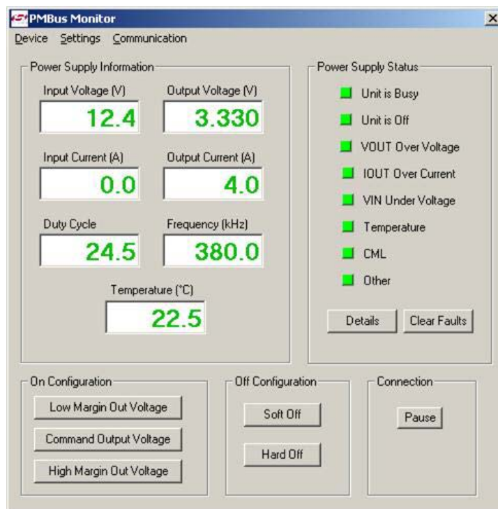
Figure 5. View of the PMBus Monitor
