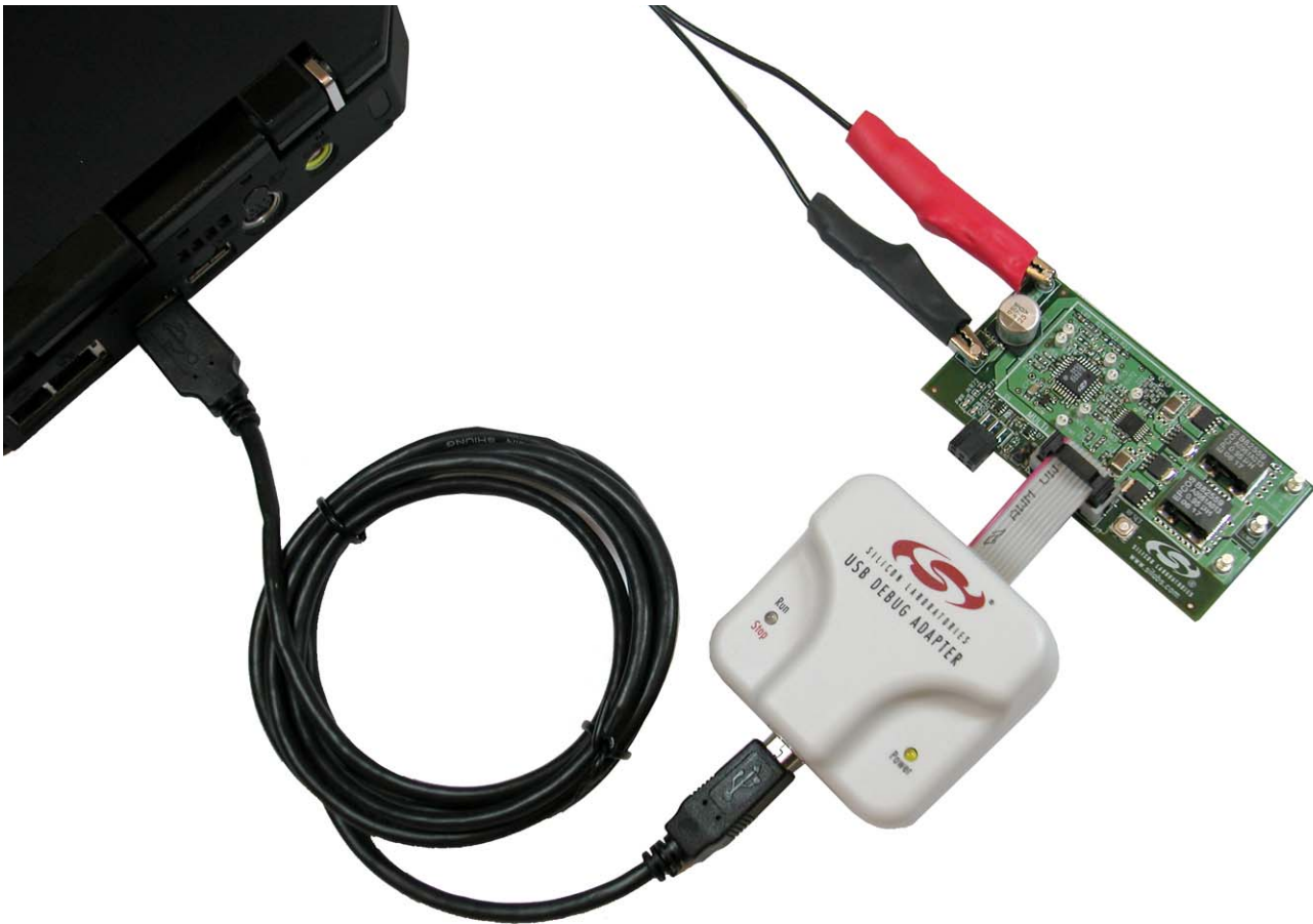
Figure 3. Overall View of the Debug Connection (Load not Connected)
