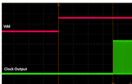
Figure 17. Startup Waveform vs. Vdd
