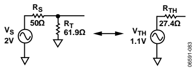
Figure 58. Calculating Thevenin Equivalent
