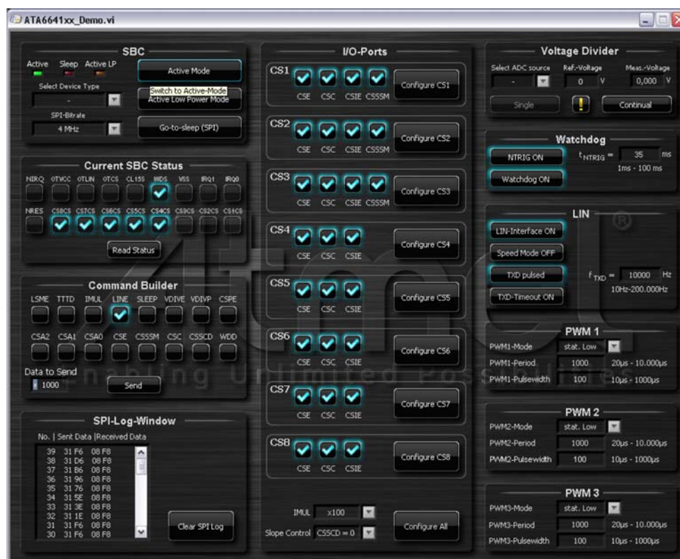
Figure 2-11. Atmel ATA664251 Demo GUI after “Active Mode” Button Is Pressed
