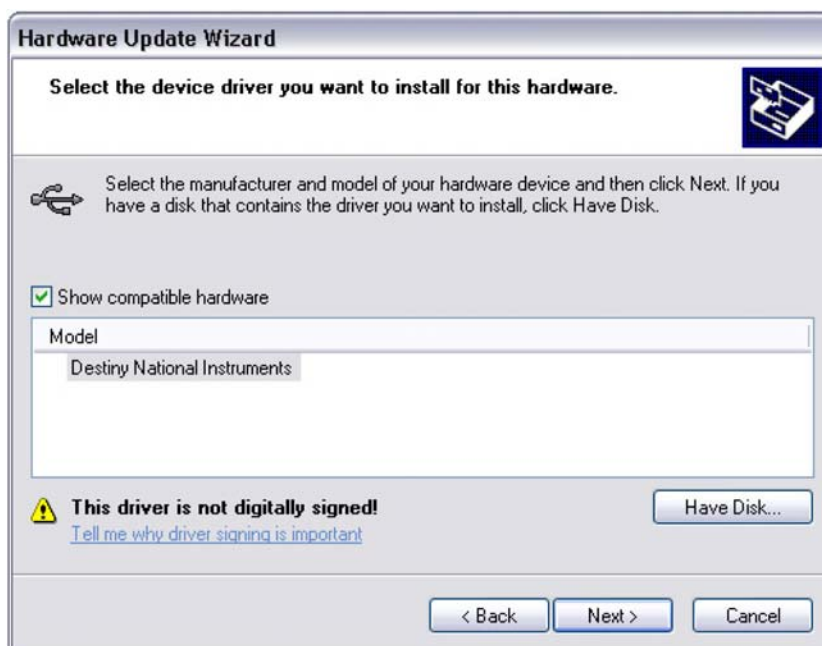
Figure 2-7. Selecting the “Destiny National Instruments” Driver
