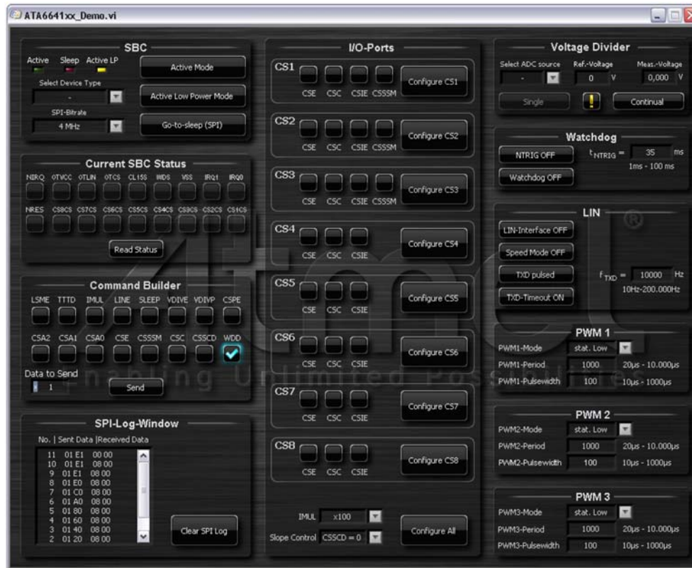
Figure 2-10. Atmel ATA664251 Demo GUI at Start-up
