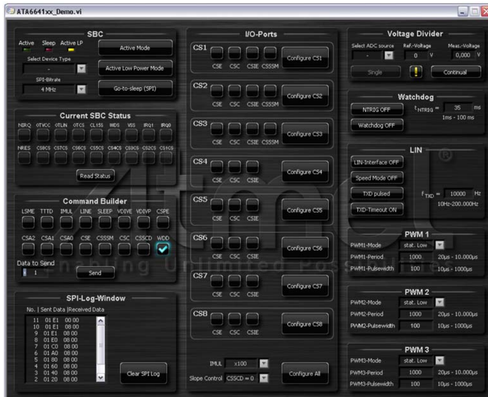
Figure 5-1. Atmel ATA664251 Demo GUI
