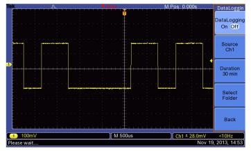
Data logging enables automatic saving of triggered waveforms.
