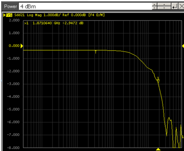
Figure 17. MHL Path SDD21 Insertion Loss Curve
