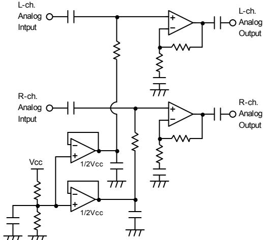
(Fig.3: Half Vcc Buffer on Single Supply Application)
