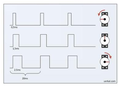
Figure 2-15 Duty Cyclone V.S. Angle
