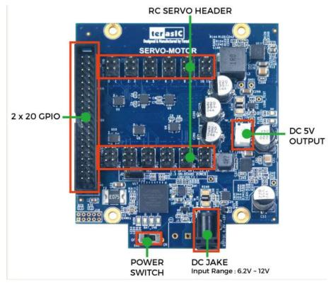
Figure 2-3 Main interface of the servo motor card
