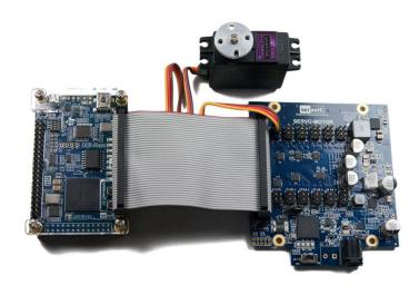
Figure 3-3 Demo Setup for DE0-Nano
