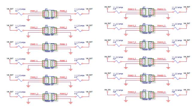
Figure 2-10 24 1x3 header for 24 servo motors
