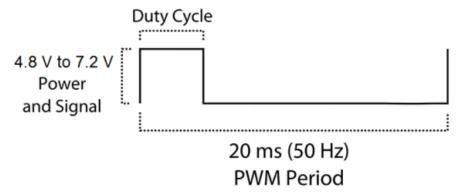
Figure 2-14 PWM Duty Cycle and Period
