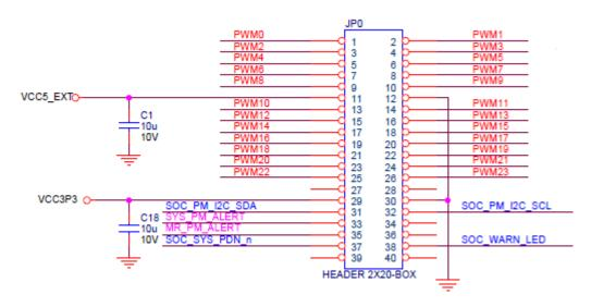
Figure 2-6 2x20 GPIO Pinout
