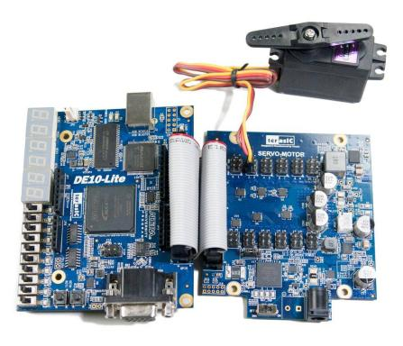
Figure 1-2 Connect the Servo Motor and Motor Card to DE10-Lite
