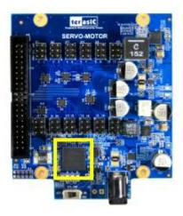
**Figure 2-12 CPLD for Power Monitor**
