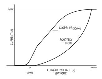
Figure 3. LTC4085 Schottky Diode vs Forward Voltage Drop
