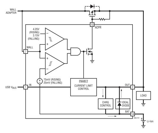
Figure 1: Simplified Block Diagram—PowerPath
