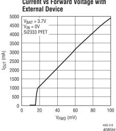
Ideal Diode Resistance and Current vs Forward Voltage with External Device
