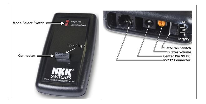
The **Mode Select Switch** has two settings; "High res" is for the High Resolution (64x32) switches/ displays and "Standard res" is for the Standard RGB switches/ displays.
