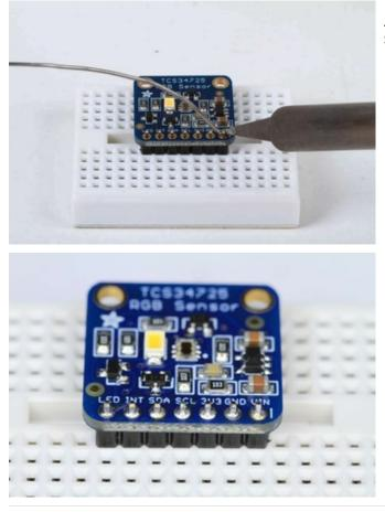
And Solder! Solder all pins to ensure good electrical contact.
