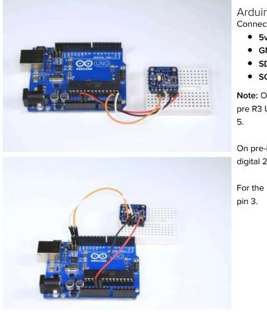
Arduino Wiring: Connect jumpers from:
