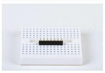
Position the header Trim the header to length if necessary and insert it (long pins down) into your breadboard.
