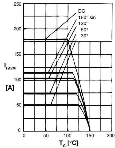
Fig. 3 Maximum forward current
