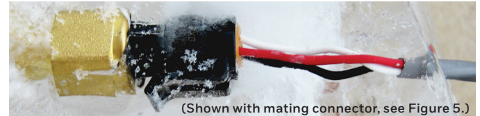
Figure 2. PX3 Series External Freeze/Thaw Resistance
