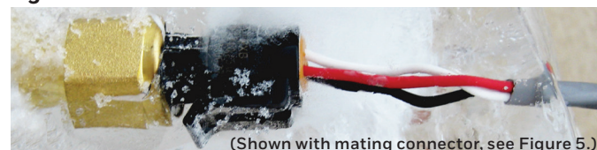
Figure 2. PX3 Series External Freeze/Thaw Resistance
