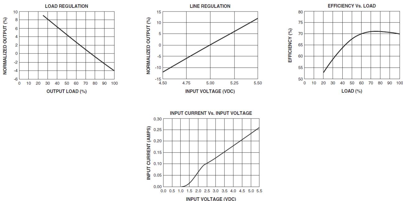
Figure 1. Typical Performance ( $T_c = 25^\circ\text{C}$ )
