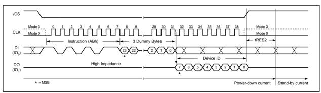
Figure 38c. Release Power-down / Device ID Instruction (SPI Mode)
