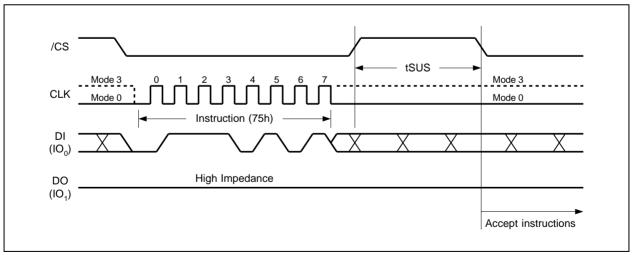
Figure 35a. Erase/Program Suspend Instruction (SPI Mode)
