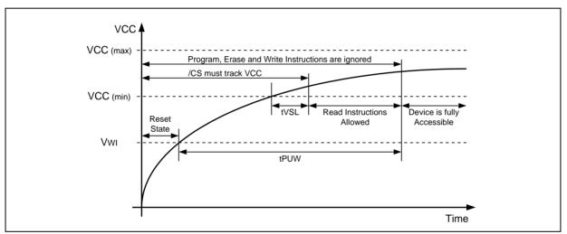
Figure 58a. Power-up Timing and Voltage Levels
