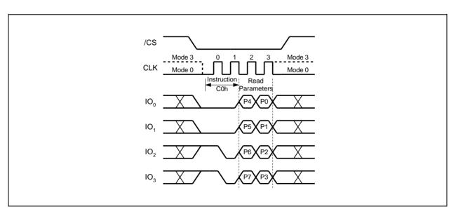
Note: 4-bytes address alignment for QPI Read: read address start from A1,A0=0,0
