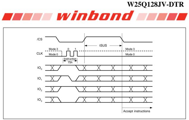
Figure 35b. Erase/Program Suspend Instruction (QPI Mode)
