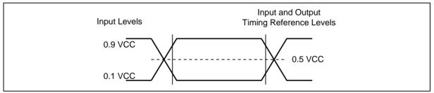
Figure 59. AC Measurement I/O Waveform
