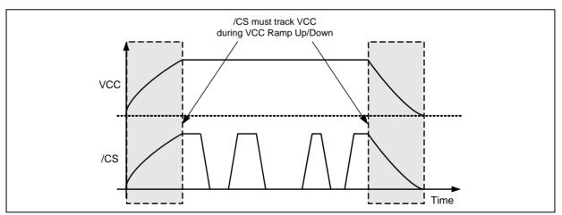
Figure 58b. Power-up, Power-Down Requirement
