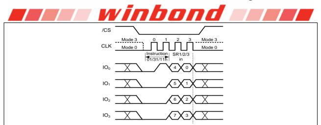
Figure 9b. Write Status Register-1/2/3 Instruction (QPI Mode)
