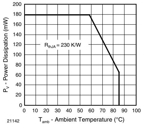
Fig. 1 - Power Dissipation Limit vs. Ambient Temperature
