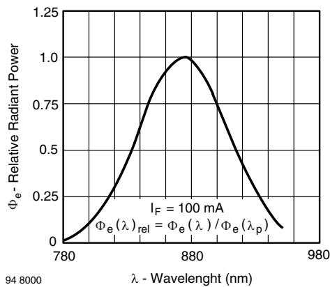
Fig. 9 - Relative Radiant Power vs. Wavelength
