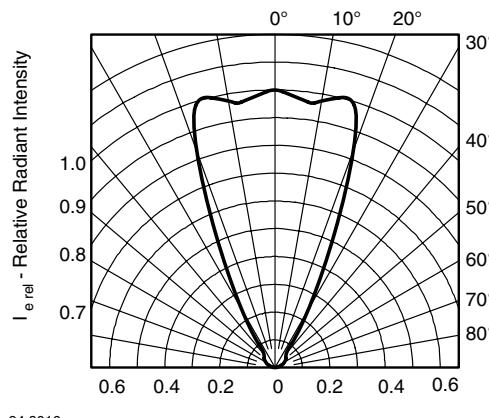
Fig. 10 - Relative Radiant Intensity vs. Angular Displacement
