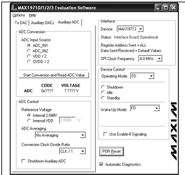
Figure 3. MAX19713 EV Kit Software Auxiliary ADC Control
