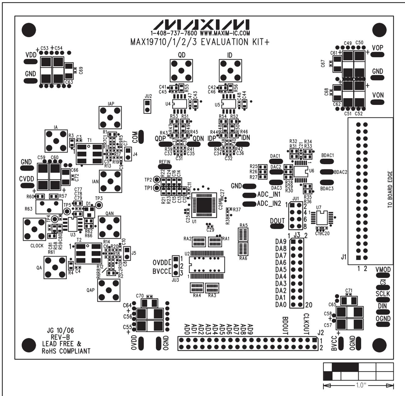
Figure 7. MAX19710-MAX19713 EV Kit Component Placement Guide—Component Side
