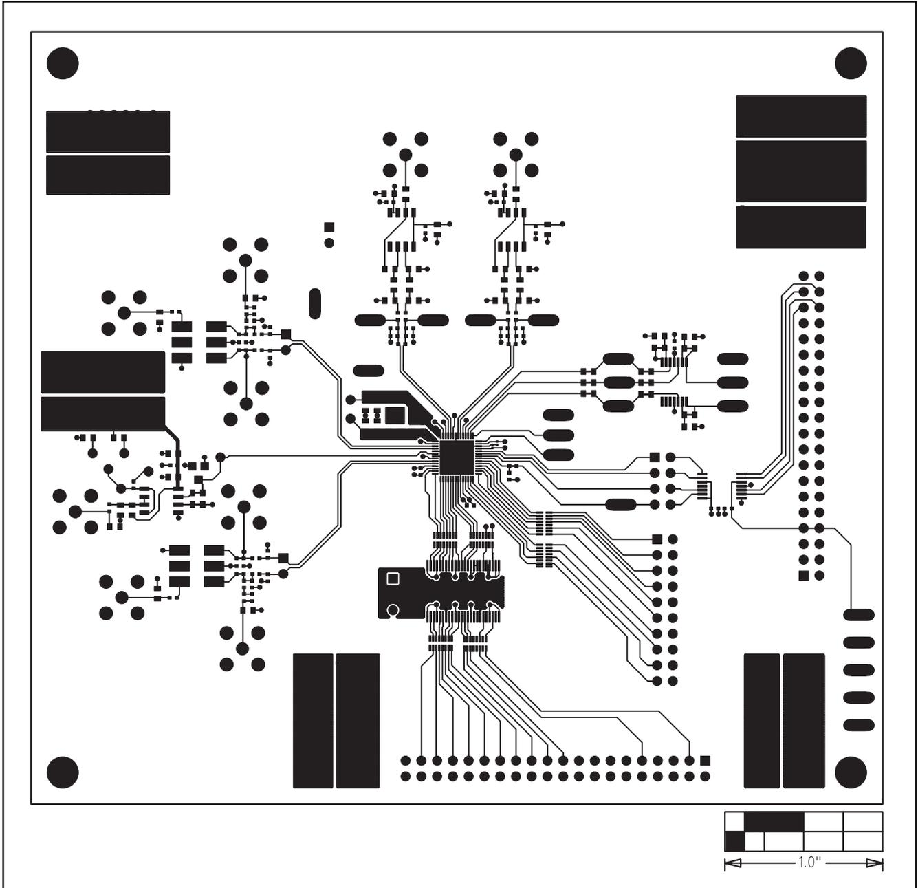
Figure 8. MAX19710-MAX19713 EV Kit PCB Layout—Component Side
