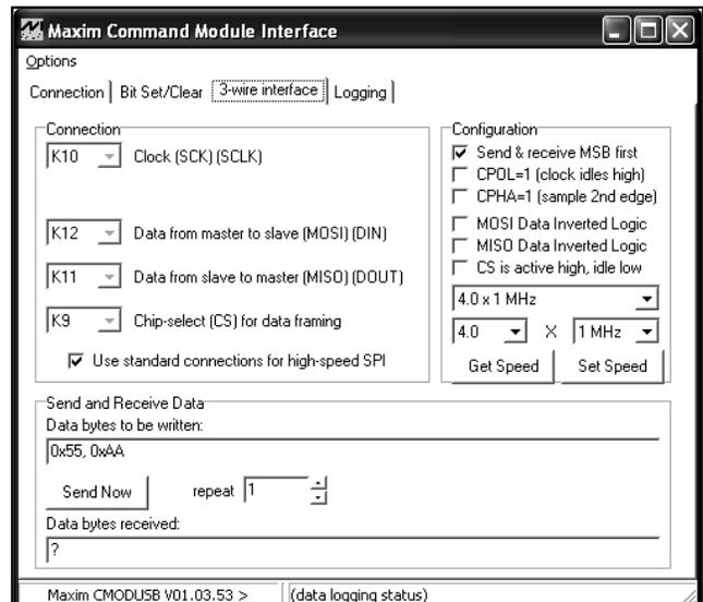
Figure 4. MAX19713 EV Kit Software 3-Wire Interface Diagnostics
