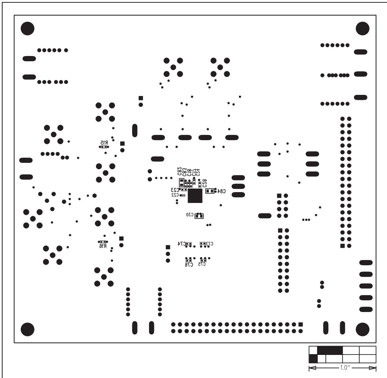
Figure 12. MAX19710-MAX19713 EV Kit Component Placement Guide—Solder Side
