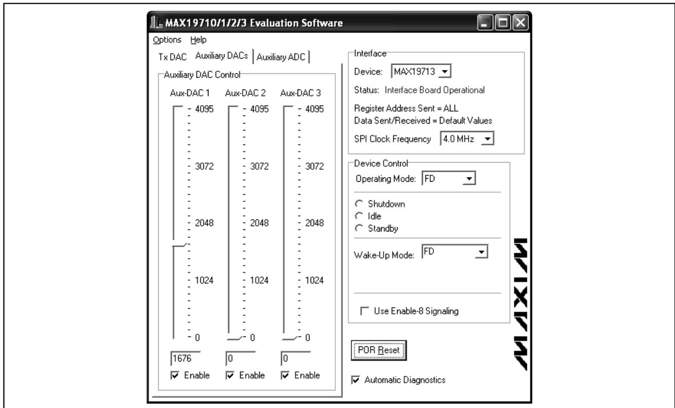
Figure 2. MAX19713 EV Kit Software Auxiliary DAC Control
