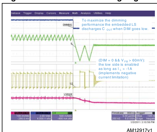
Figure 28. LED current falling edge
