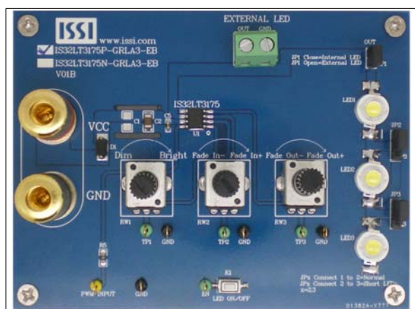
Figure 1: Photo of IS32LT3175N/P Evaluation Board
