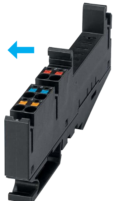
18plus-AM connection module terminal 2.1/2.2 (LINE +), terminal 3.1/3.2 (0 V), terminal 4.1/4.2 (FE)
