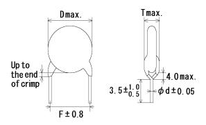
Note) The mark '\*' of lead code differ from lead spacing(F) and lead diameter(d).
