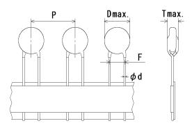
Note) The mark '\*' of lead code differ from lead spacing(F), lead diameter(d) and pitch of component(P). Please see the following list or taping specification about details.
